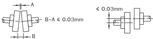
Figure 1: Coupling alignment
